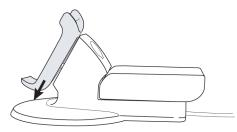
6. Align the slots and the USB port on the BlackBerry<sup>®</sup> C-Series Battery Charger with the tabs and the USB port on the base of the BlackBerry Power Station.
